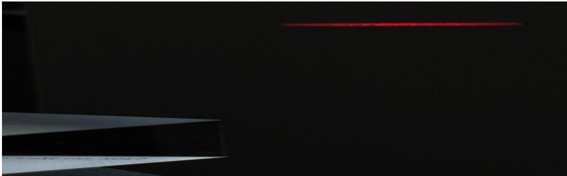
Extremely elongated Gaussian beam (with a 30  $\mu\text{m}$  height, at its center, and a 60000  $\mu\text{m}$  width) used as illumination source in the NSLI. The last stage in the multiple-prism beam expansion array is shown at the lower left. Note: the beam in this image appears much higher due to saturation in the detector array capturing the image. This type of extremely elongated coherent illumination, first demonstrated in 1987, has also become known as 'light sheet illumination.'
